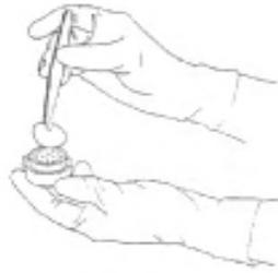
Figure 6-14 Placing Filter Membrane onto Filter Holder
