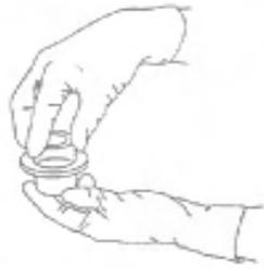
Figure 6-15 Securing Top of Filter Holder onto Bottom
